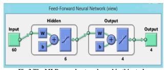
**Fig.3 The MLP neural network used in this study.** One of the key parameters in the MLP neural network is the number of neurons in hidden layers. In order to find out the number of suitable neurons in each hidden layer, the hidden layers were raised from 1 to 13 while the categorization percentage was calculated. The highest value was for six neurons in the hidden layer. Figure 4 illustrates the results of neuron modification in the hidden layer.
