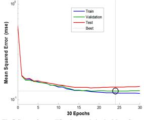
Fig.5 Curves for modification made in the Mean Squared Error (MSE) throughout the training procedure.
